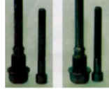
4. Alkaline zinc-nickel-plated fasteners. Right is as plated; left after 136 hrs salt spray and one hr heat treatment at 250F.
